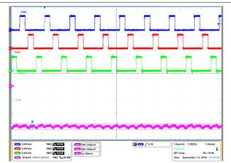
Figure 6-3. 3-phase switching ripple at Input Voltage = 5 V, Load current = 50A, Switching Frequency = 800kHz. Persistence mode.
