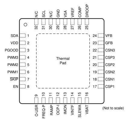
Figure 5-1. RHB Package 32-Pin QFN (Top View)
