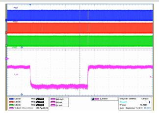
Figure 6-8. Load transient with a droop of  $0.6m\Omega$  load-line slope. Load transient = 14A to 50A. Persistence mode
