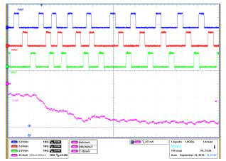
Figure 6-6. Load transient with a droop of  $0.6m\Omega$  load-line slope. Load transient = 14A to 50A. Single mode.
