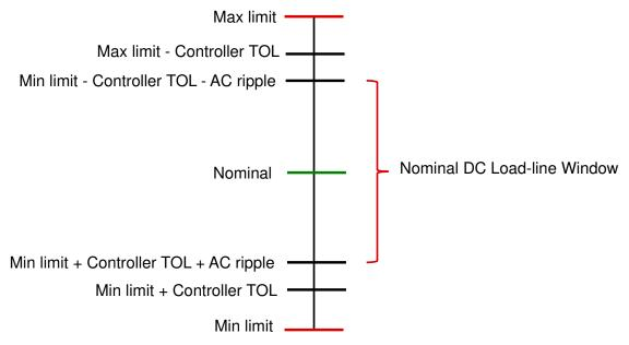
Figure 8-2. Determination of Nominal DC Load-line window
