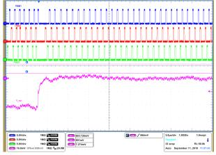
Figure 6-5. Load transient with a droop of  $0.6m\Omega$  load-line slope. Load transient = 36A to 0A. Single mode.
