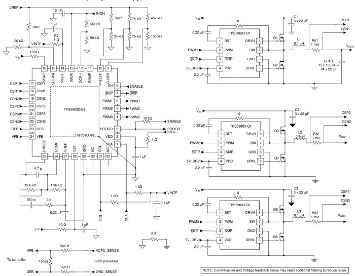
Figure 8-1. 3-Phase D-CAP+™, Step-Down Application with Power Stages
