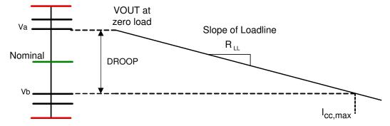
Figure 8-3. Determination of the Slope of the Load-line
