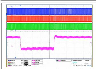
Figure 6-7. Load transient with a droop of  $0.6m\Omega$  load-line slope. Load transient = 0A to 36A. Persistence mode
