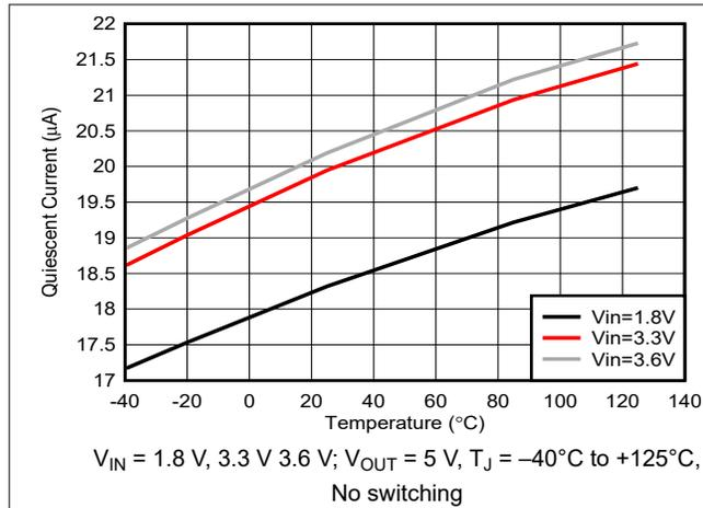
Figure 6-7. Quiescent Current into VIN vs Temperature
