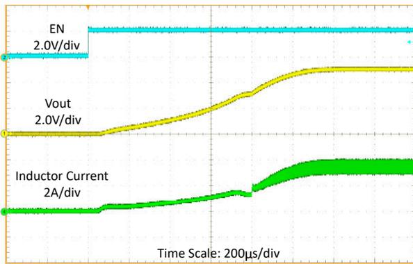
$V_{IN} = 3.3\text{ V}$ ,  $V_{OUT} = 5\text{ V}$ ,  $2.5\text{-}\Omega$  resistance load
