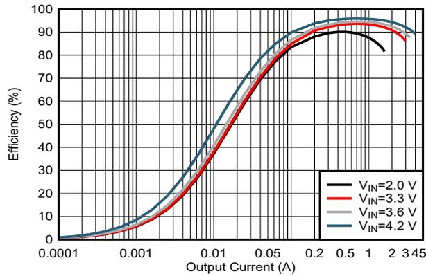
$V_{IN} = 2.0\text{ V}, 3.3\text{ V}, 3.6\text{ V}, 4.2\text{ V}$ ;  $L = 0.47\ \mu\text{H}$ , PWM Mode
