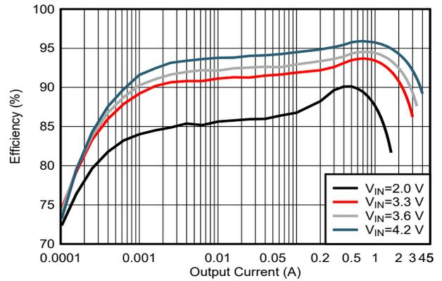
$V_{IN} = 2.0\text{ V}, 3.3\text{ V}, 3.6\text{ V}, 4.2\text{ V}$ ;  $L = 0.47\ \mu\text{H}$ , Auto PFM Mode
