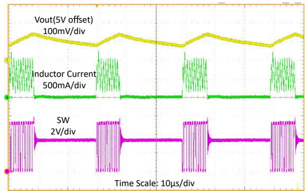
$V_{IN} = 3.3\text{ V}$ ,  $V_{OUT} = 5\text{ V}$ ,  $I_{OUT} = 100\text{ mA}$
