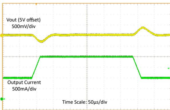
$V_{IN} = 3.3\text{ V}$ ,  $V_{OUT} = 5\text{ V}$ ,  $I_{OUT} = 1\text{ A to } 2\text{ A}$  with  $20\text{-}\mu\text{s}$  slew rate
