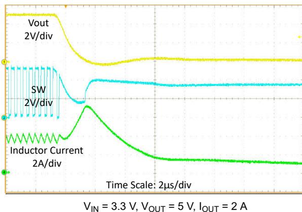
**Figure 8-10. Output Short Protection (Entry)**
