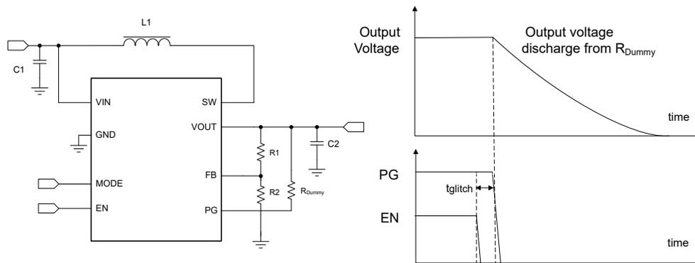
**Figure 7-1. Implement Output Discharge by PG function**
