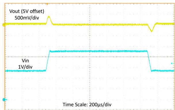
$V_{IN} = 2.7\text{ V to } 4.5\text{ V}$  with  $20\text{-}\mu\text{s}$  slew rate,  $V_{OUT} = 5\text{ V}$ ,  $I_{OUT} = 2\text{ A}$
