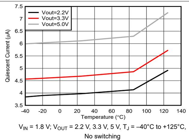
Figure 6-8. Quiescent Current into VOUT vs Temperature
