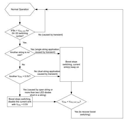
Figure 7. V<sub>IFBX</sub> OVP Protection Action
