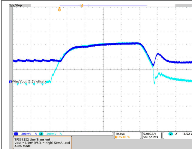
Figure 10-16. TPS61281D Forced Pass-Through to Boost Mode Transition
