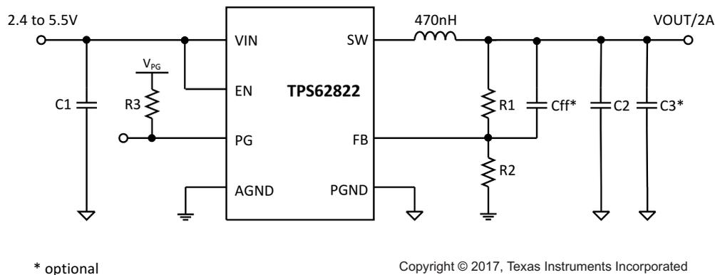
**Figure 7. A typical 2.4 to 5.5-V, 2-A Power Supply**
