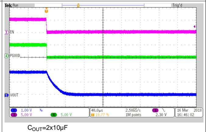
Figure 43. Active Output Discharge at load 1.8-Ohm
