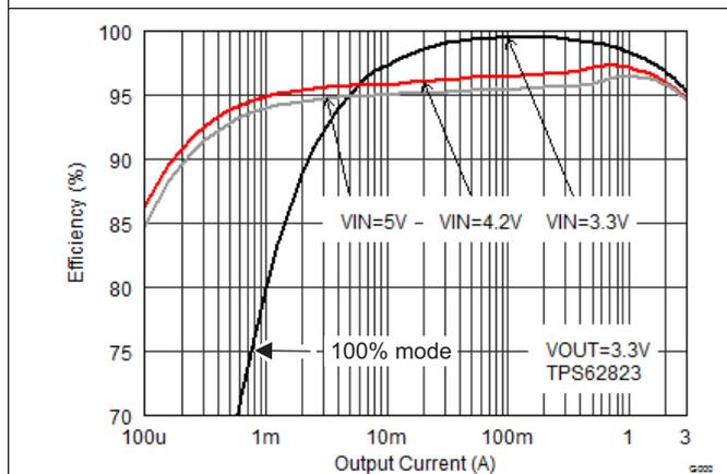
Figure 12. Efficiency TPS62823 at VOUT=3.3V
