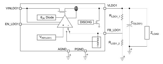
Figure 19. LDO Block Diagram and Output Voltage Setting
