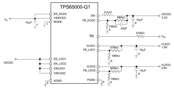
Figure 23. Typical TPS65000-Q1 Application Schematic
