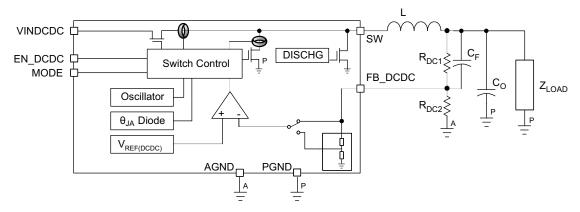
Figure 16. DC-DC Converter Block Diagram and Output Voltage Setting
