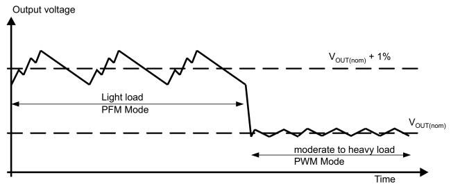
Figure 17. PFM Voltage Positioning
