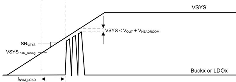
Figure 7-4. VSYS Slow Ramp With FSD and MASK\_RETRY\_COUNT\_ON\_FIRST\_PU = '0'
