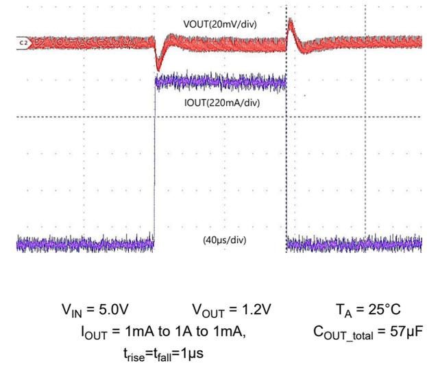
**Figure 6-4. BUCK Load-Step Response - High Bandwidth, Forced PWM**
