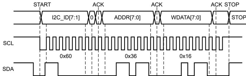
**Figure 7-12. I<sup>2</sup>C Write Cycle**
