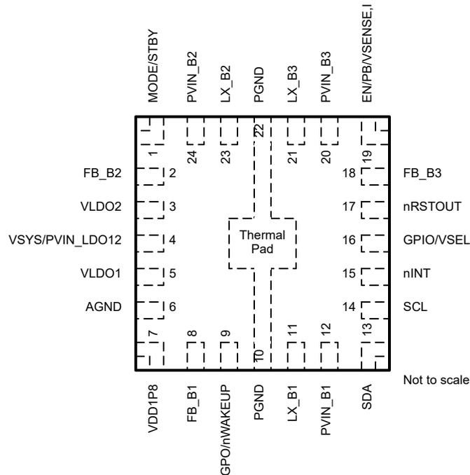
Figure 5-1. TPS65214 VAF Package, 24-pin QFN (Top View)
