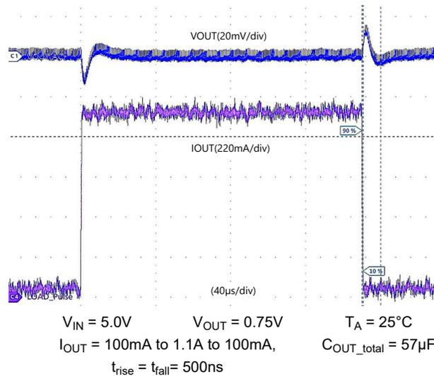
**Figure 6-3. BUCK Load-Step Response - High Bandwidth, Forced PWM**
