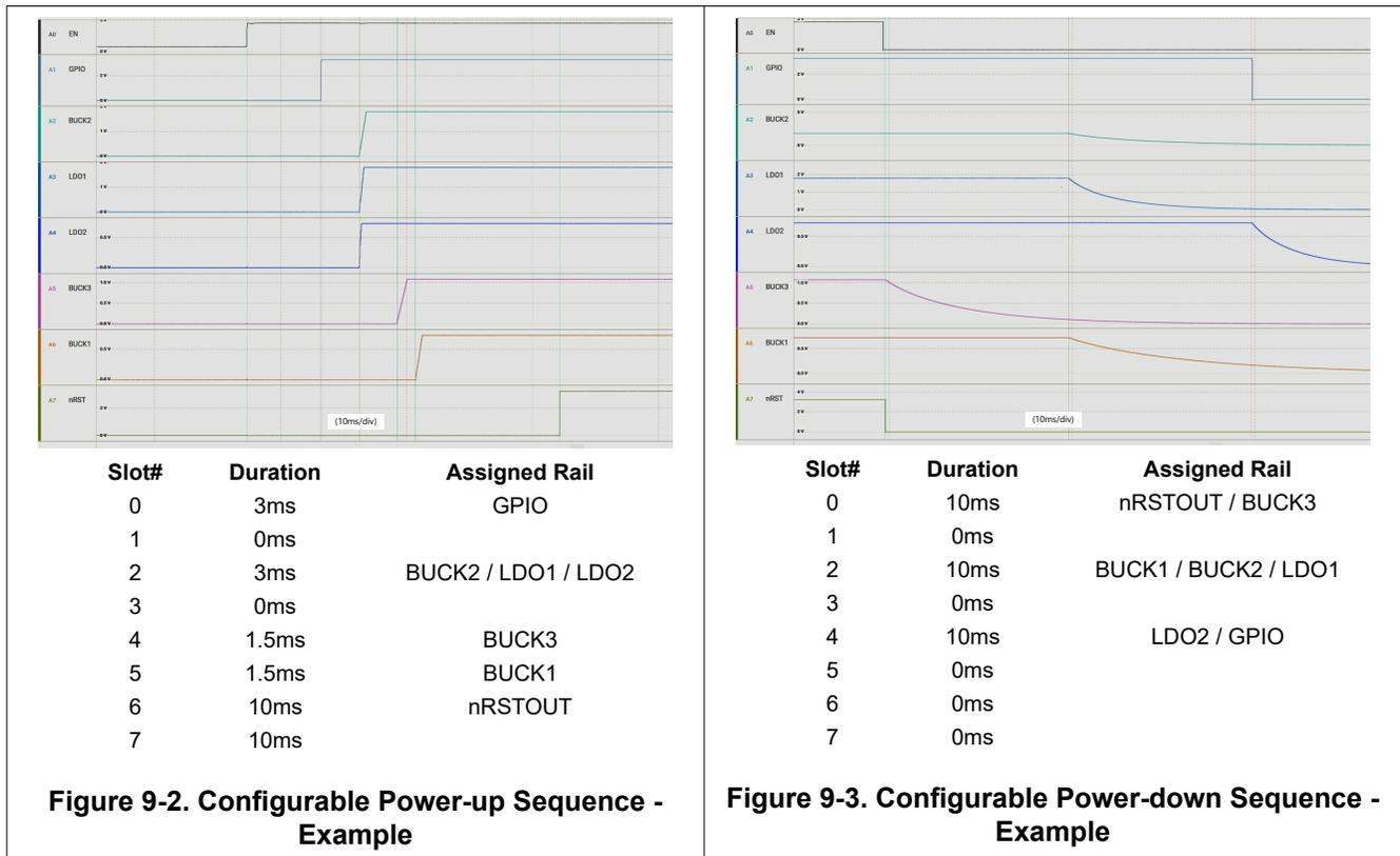
**Figure 9-2. Configurable Power-up Sequence - Example**
