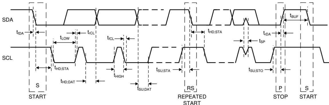
Figure 7-10. I<sup>2</sup>C-Compatible Timing
