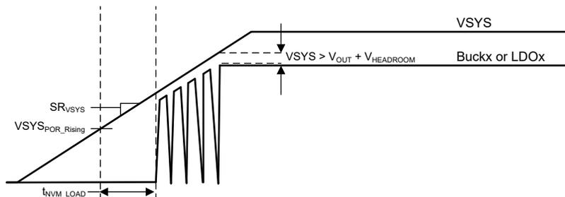
Figure 7-5. VSYS Slow Ramp With FSD and MASK\_RETRY\_COUNT\_ON\_FIRST\_PU = '1'
