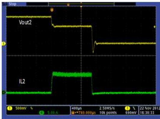
Figure 29. Over Current Protection, Buck 2
