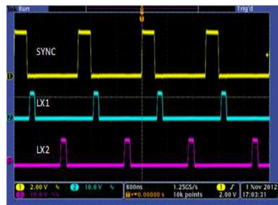
Figure 32. Synchronization at 500 kHz
