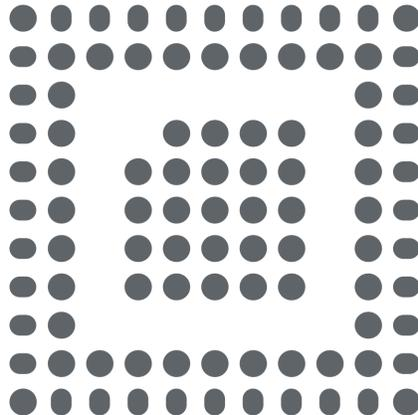
**Figure 11-5. Example Footprint with Oval Pads**
