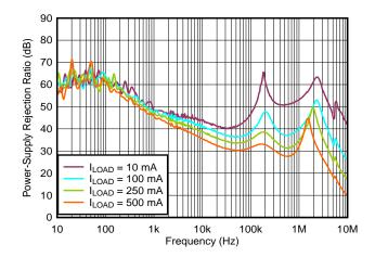
$V_{IN}$  = 3.8 V,  $V_{OUT}$  = 3.3 V,  $C_{OUT}$  = 2.2  $\mu F$
