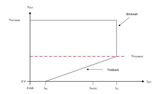
Figure 43. Foldback Current Limit
