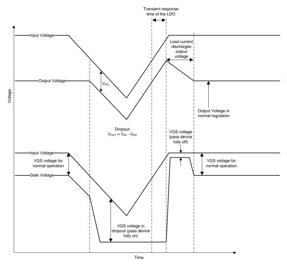
Figure 46. Line Transients From Dropout
