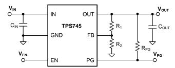
Figure 44. Adjustable Operation
