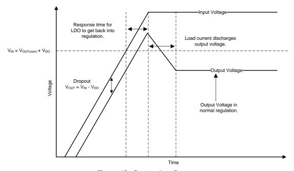
Figure 45. Startup Into Dropout
