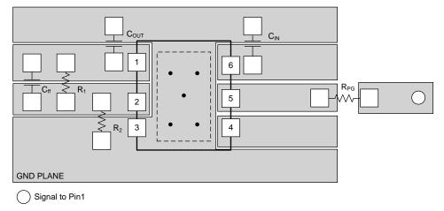
Figure 50. DRV Package Layout Example
