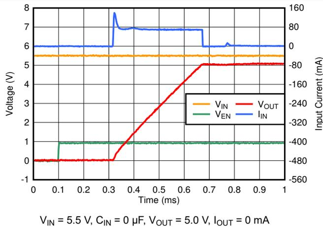
Figure 6-33. Startup Inrush Current With  $C_{OUT} = 4.7\text{ }\mu\text{F}$
