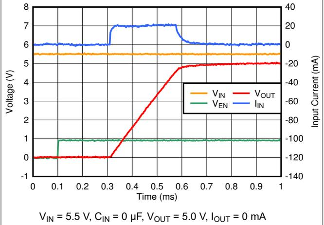
Figure 6-32. Startup Inrush Current With  $C_{OUT} = 1\text{ }\mu\text{F}$
