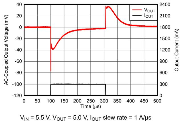
Figure 6-18.  $I_{OUT}$  Transient From 1 mA to 300 mA
