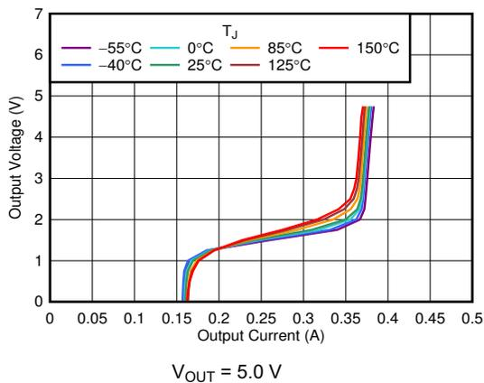
Figure 6-15. Foldback Current Limit vs  $I_{OUT}$  and Temperature
