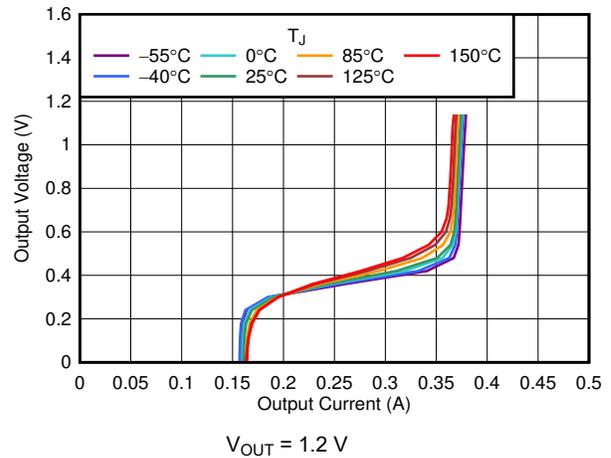
Figure 6-14. Foldback Current Limit vs  $I_{OUT}$  and Temperature
