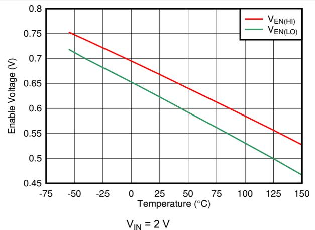
Figure 6-12.  $V_{EN(HI)}$  and  $V_{EV(LO)}$  Threshold vs Temperature
