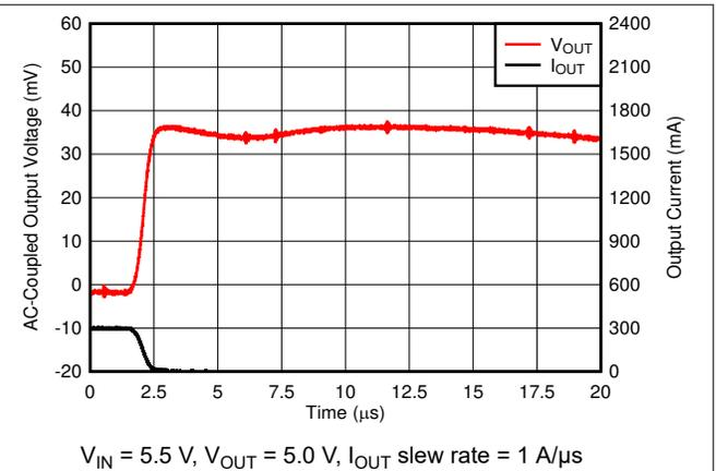
**Figure 6-20.  $I_{OUT}$  Transient From 300 mA to 1 mA**
