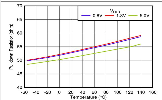
Figure 6-41. Pulldown Resistor vs Temperature and  $V_{OUT}$
