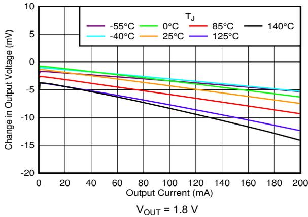
**Figure 6-31. Load Regulation vs  $V_{IN}$  and Temperature**
