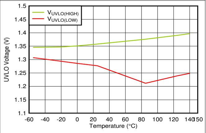
Figure 6-40. UVLO Rising and Falling Threshold vs Temperature
