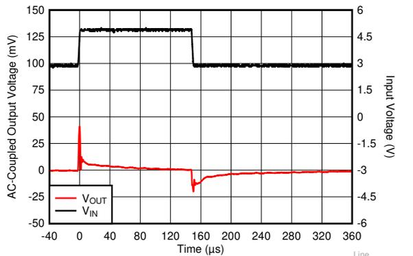
$V_{OUT} = 1.8\text{ V}$ ,  $I_{OUT} = 200\text{ mA}$ ,  $C_{OUT} = 1\text{ }\mu\text{F}$ , slew rate =  $1\text{ V}/\mu\text{s}$
