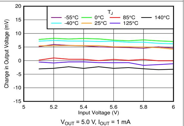
Figure 6-28. Line Regulation vs  $V_{IN}$  and Temperature
