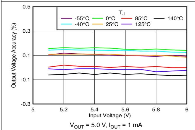
Figure 6-29. Output Accuracy vs  $V_{IN}$  and Temperature
