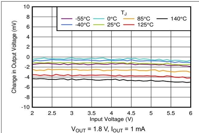
Figure 6-25. Line Regulation vs  $V_{IN}$  and Temperature
