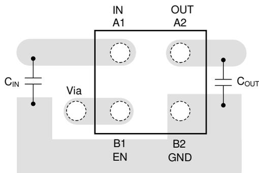
**Figure 8-8. Layout Example for the YCH Package**
