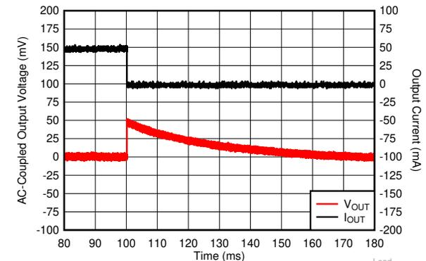
$V_{OUT} = 1.8\text{ V}$ ,  $V_{IN} = 2.8\text{ V}$ ,  $C_{OUT} = 1\text{ }\mu\text{F}$ ,  $t_r = t_f = 1\text{ }\mu\text{s}$
