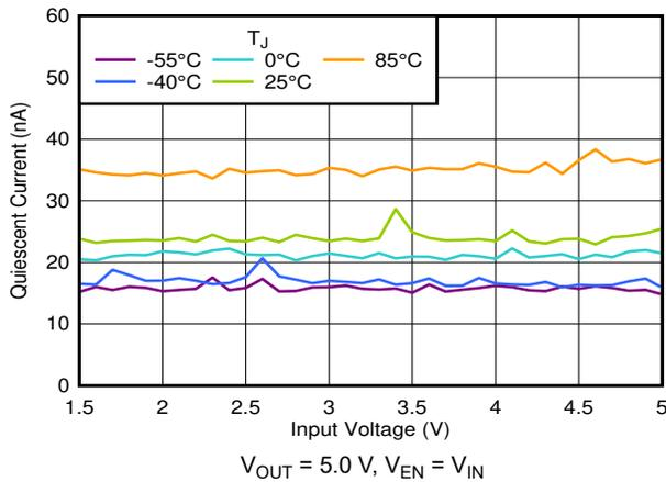
Figure 6-7.  $I_Q$  in Dropout vs  $V_{IN}$  and Temperature
