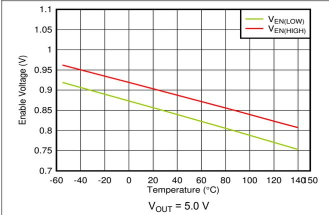
Figure 6-39. EN High and Low Threshold vs Temperature
