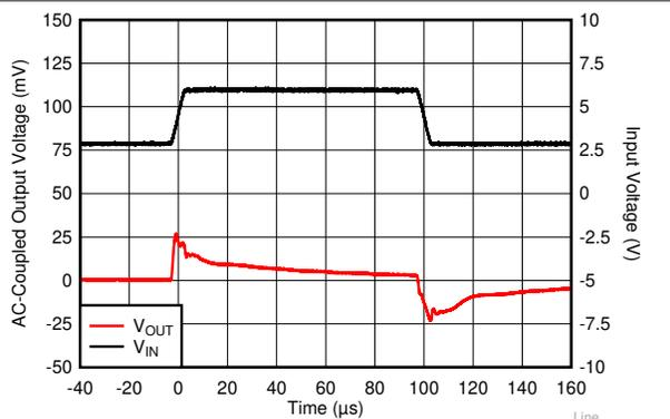
$V_{OUT} = 1.8\text{ V}$ ,  $I_{OUT} = 200\text{ mA}$ ,  $C_{OUT} = 1\text{ }\mu\text{F}$ , slew rate =  $1\text{ V}/\mu\text{s}$
