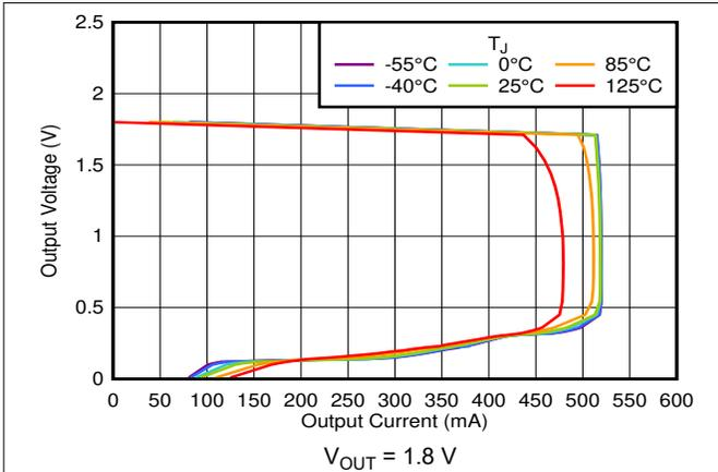
Figure 6-37. Foldback Current Limit vs  $I_{OUT}$  and Temperature
