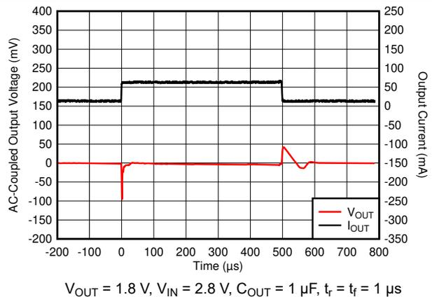
Figure 6-12.  $I_{OUT}$  Transient From 1 mA to 50 mA
