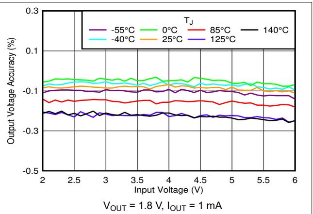
Figure 6-26. Output Accuracy vs  $V_{IN}$  and Temperature
