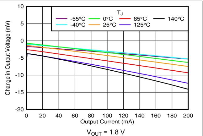
**Figure 6-32. Load Regulation vs  $V_{IN}$  and Temperature**
