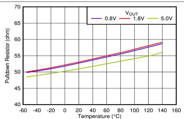
**Figure 6-42. Pulldown Resistor vs Temperature and  $V_{OUT}$**
