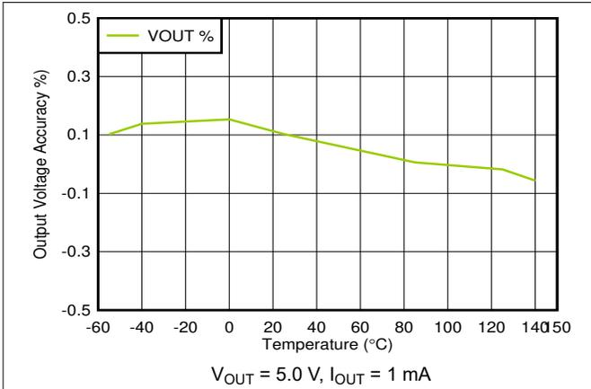
**Figure 6-31. Output Accuracy vs Temperature**
