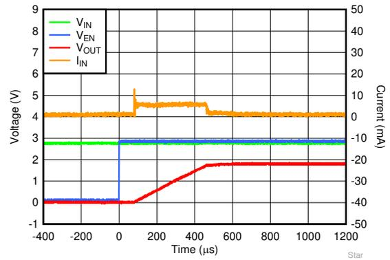
$V_{OUT} = 1.8\text{ V}$ ,  $I_{OUT} = 0\text{ mA}$
