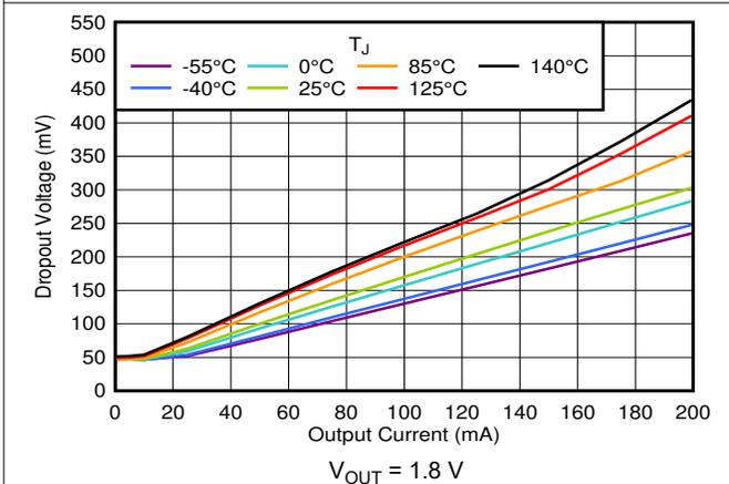
**Figure 6-33. Dropout vs  $I_{OUT}$  and Temperature**
