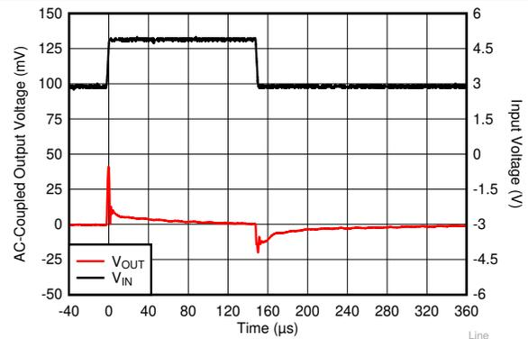
$V_{OUT} = 1.8\text{ V}$ ,  $I_{OUT} = 200\text{ mA}$ ,  $C_{OUT} = 1\ \mu\text{F}$ , slew rate =  $1\text{ V}/\mu\text{s}$
