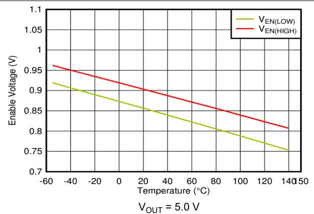
**Figure 6-40. EN High and Low Threshold vs Temperature**
