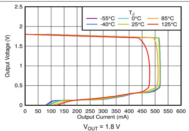
**Figure 6-38. Foldback Current Limit vs  $I_{OUT}$  and Temperature**
