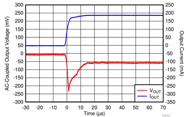
$V_{OUT} = 1.8\text{ V}$ ,  $V_{IN} = 2.8\text{ V}$ ,  $C_{OUT} = 1\ \mu\text{F}$ ,  $t_r = t_f = 1\ \mu\text{s}$
