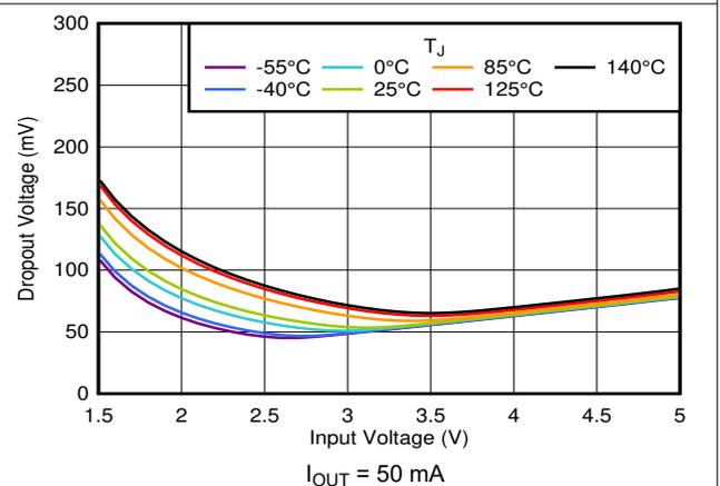
**Figure 6-36. Dropout vs  $V_{IN}$  and Temperature**
