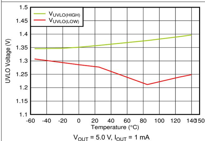
**Figure 6-41. UVLO Rising and Falling Threshold vs Temperature**
