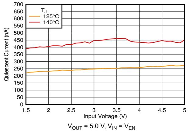
Figure 6-8.  $I_Q$  in Dropout vs  $V_{IN}$  and Temperature
