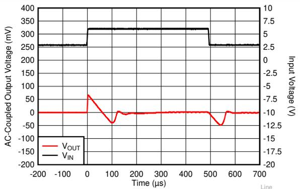
$V_{OUT} = 1.8\text{ V}$ ,  $I_{OUT} = 1\text{ mA}$ ,  $C_{OUT} = 1\ \mu\text{F}$ , slew rate =  $1\text{ V}/\mu\text{s}$
