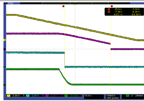
CH1: V_{(SUPPLY)} CH2: V_{(FAULT)} CH3: V_{(REF)} CH4: I_{(OUT8)}
