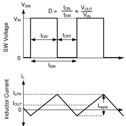
FPWM mode Continuous Conduction (CCM) is possible even if  $I_{OUT}$  is less than half of  $I_{ripple}$ .
