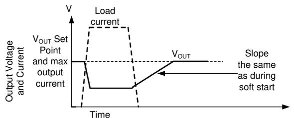
Whether output voltage falls due to high load or low input voltage, after the condition that causes output to fall below the setpoint is removed, output climbs at the same speed as during start-up. Even though hiccup does not trigger due to dropout, hiccup can, in principal, be triggered during recovery if output voltage is below 0.4 times output the setpoint for more than 128 clock cycles during recovery.
