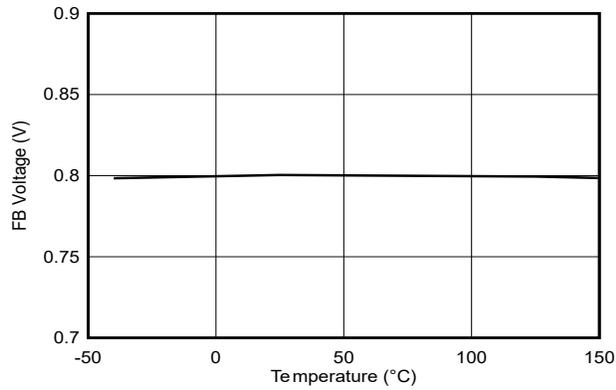
**Figure 6-1. Feedback Voltage**
