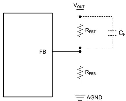
**Figure 7-1. Setting Output Voltage of Adjustable Versions**
