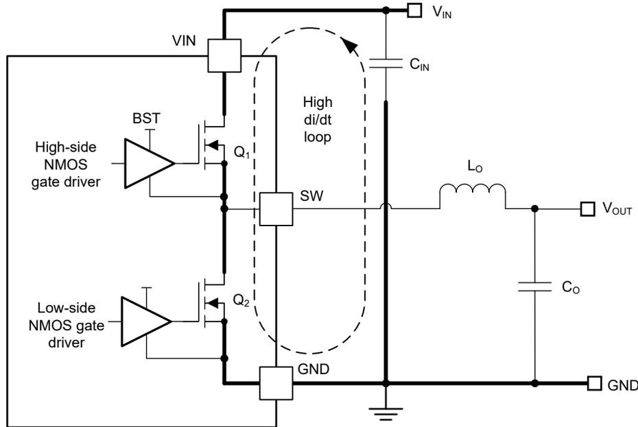
**Figure 8-19. Current Loops With Fast Edges**
