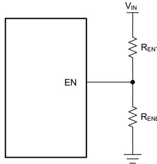
**Figure 7-2.  $V_{IN}$  UVLO Using the EN Pin**
