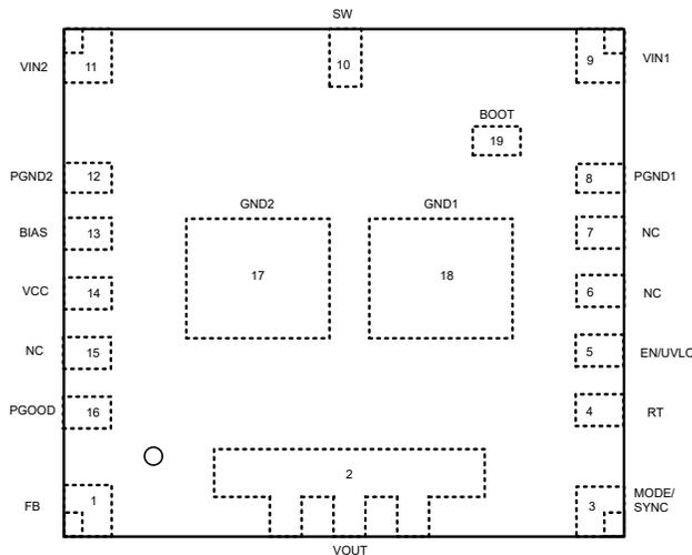
**Figure 5-1. 19-Pin VCG, QFN-FCMOD Package (Top View)**
