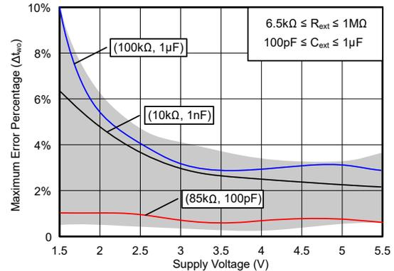
Figure 5-23. Maximum Output Pulse Width Error (Absolute Value) Across Supply Voltage
