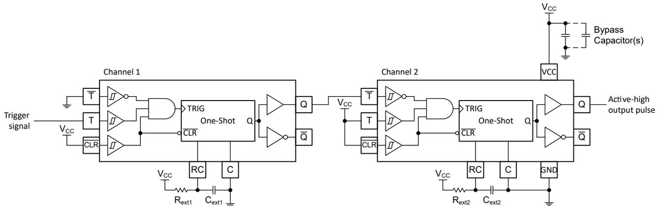
Figure 8-4. Delayed Pulse Generation Schematic Using the TPUL2G122x
