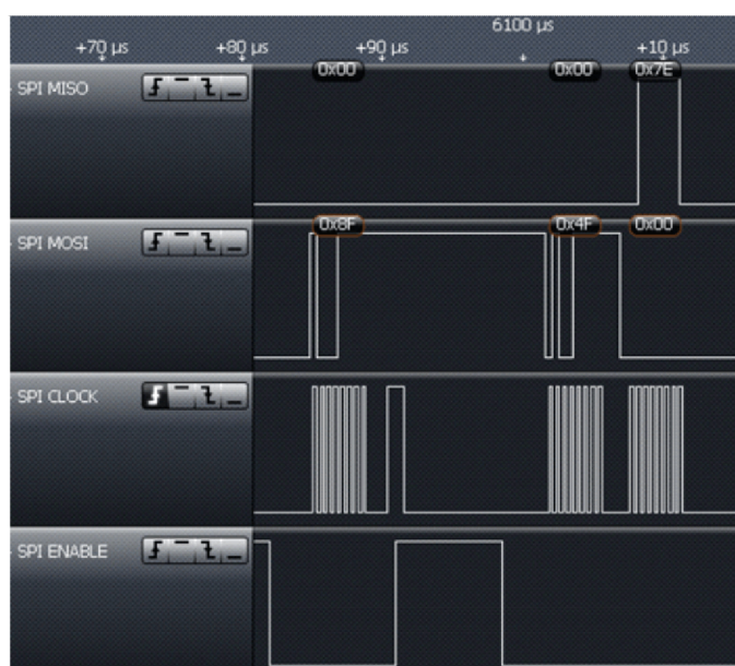
Figure 6-25. Reset FIFO and Read RSSI
