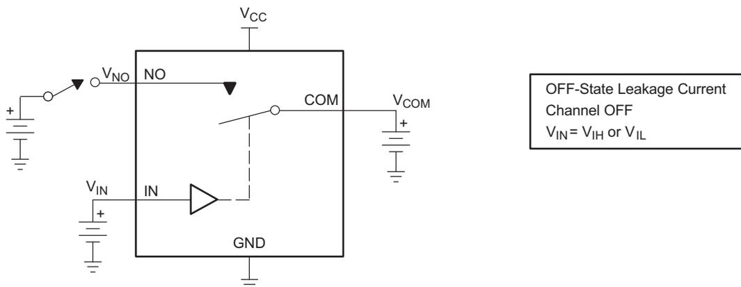
Figure 17. OFF-State Leakage Current ( $I_{COM(OFF)}$ ,  $I_{NO(OFF)}$ )
