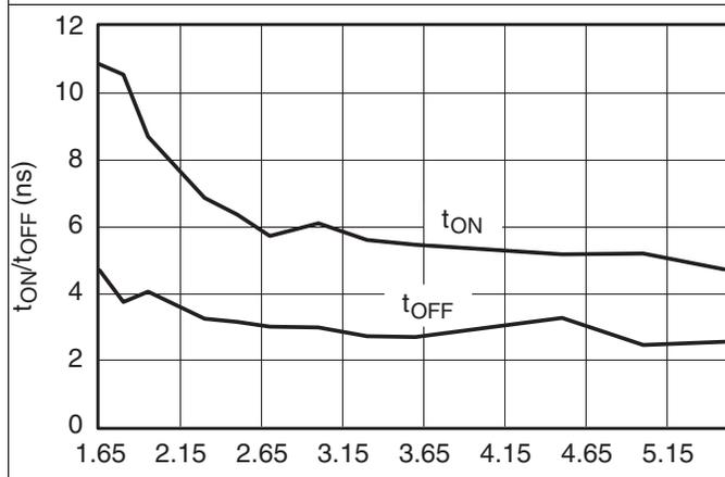
Figure 9. tON and tOFF vs VCC
