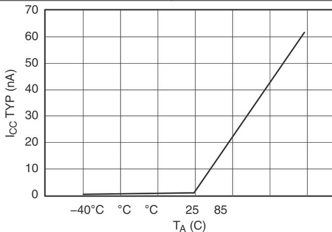
Figure 15. Power-Supply Current vs Temperature ( $V_{CC} = 5\text{ V}$ )
