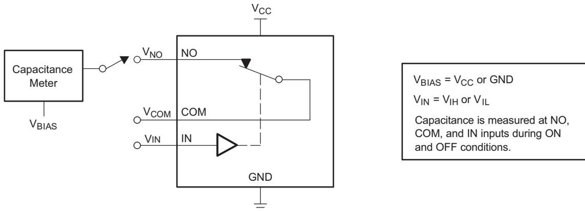
Figure 19. Capacitance ( $C_{IN}$ ,  $C_{COM(OFF)}$ ,  $C_{COM(ON)}$ ,  $C_{NO(OFF)}$ ,  $C_{NO(ON)}$ )
