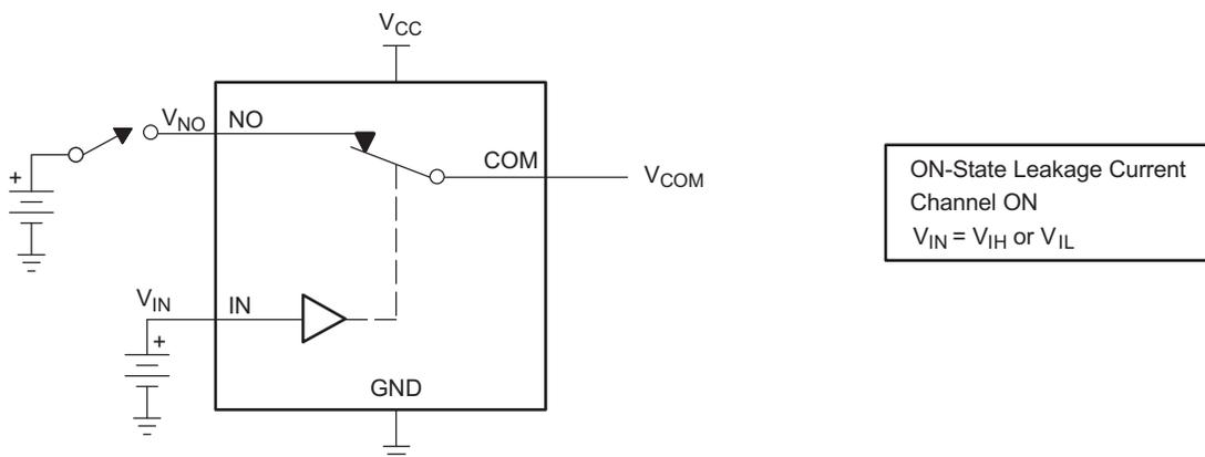
Figure 18. ON-State Leakage Current ( $I_{COM(ON)}$ ,  $I_{NO(ON)}$ )
