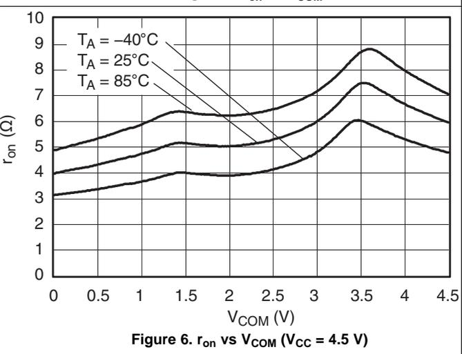
Figure 6.  $r_{on}$  vs  $V_{COM}$  ( $V_{CC} = 4.5$  V)
