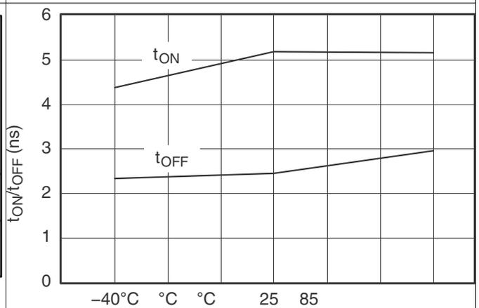
Figure 10. tON and tOFF vs Temperature (VCC = 5 V)
