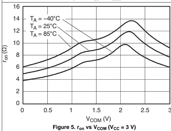
Figure 5.  $r_{on}$  vs  $V_{COM}$  ( $V_{CC} = 3$  V)
