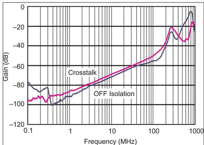
Figure 13. OFF Isolation and Crosstalk ( $V_{CC} = 5\text{ V}$ )
