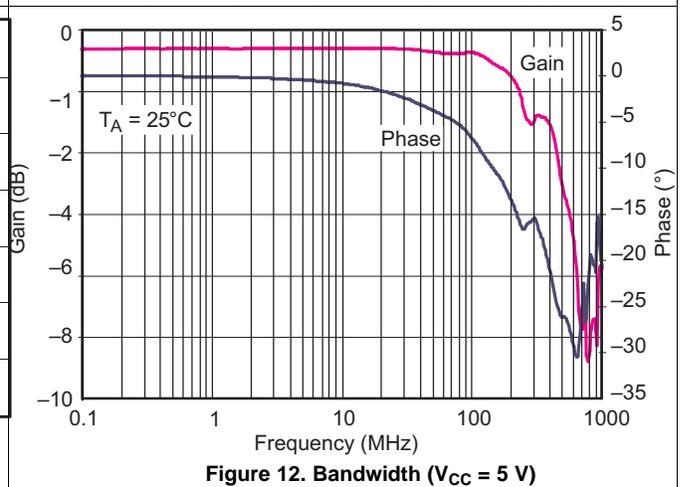
Figure 12. Bandwidth (VCC = 5 V)
