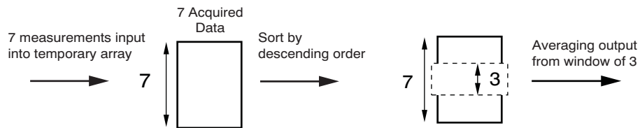
Figure 28. MAV Filter Operation (Patent Pending)
