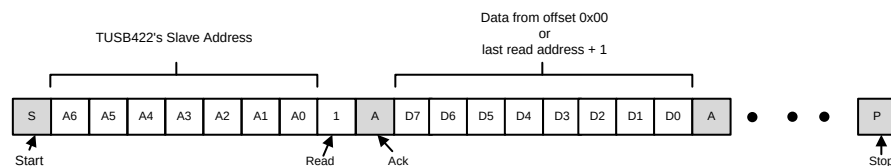
Figure 7. I2C Read Without Repeated Start
