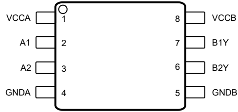
Figure 4-4. TXGx020DDF 8-Pin SOT and TXGx020D 8-pin SOIC Top View
