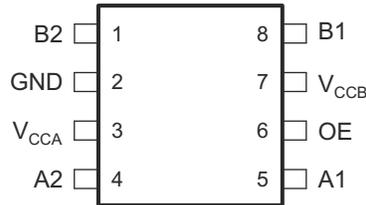
**Figure 4-1. DCU Package 8-Pin VSSOP Top View**
