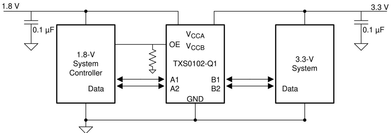
**Figure 9-1. Application Schematic**
