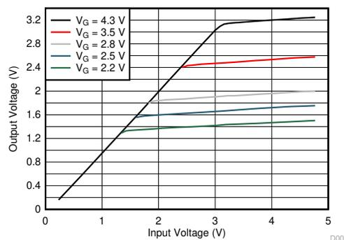
Transfer Characteristics of an N-Channel Transistor
