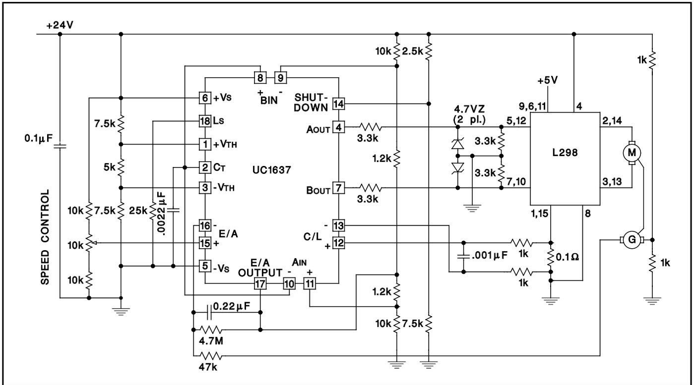
Figure 7. Bi-Directional Motor Drive with Speed Control Power-Amplifier
