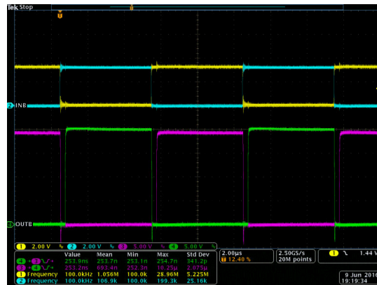
Figure 8-5. Bench Test Waveform for INA/B and OUTA/B
