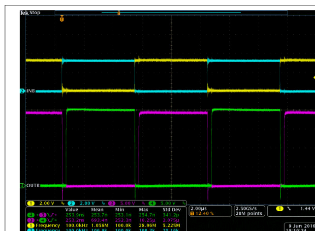
Figure 8-5. Bench Test Waveform for INA/B and OUTA/B
