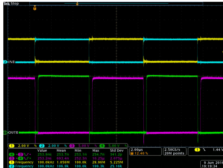
Figure 8-5. Bench Test Waveform for INA/B and OUTA/B
