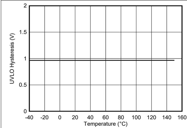
Figure 5-17. VDD 12-V UVLO Hysteresis vs Temperature
