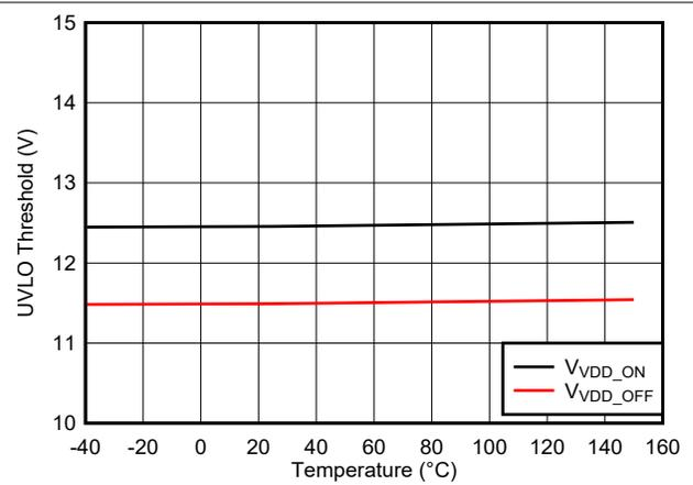
Figure 5-16. VDD 12-V UVLO Threshold vs Temperature
