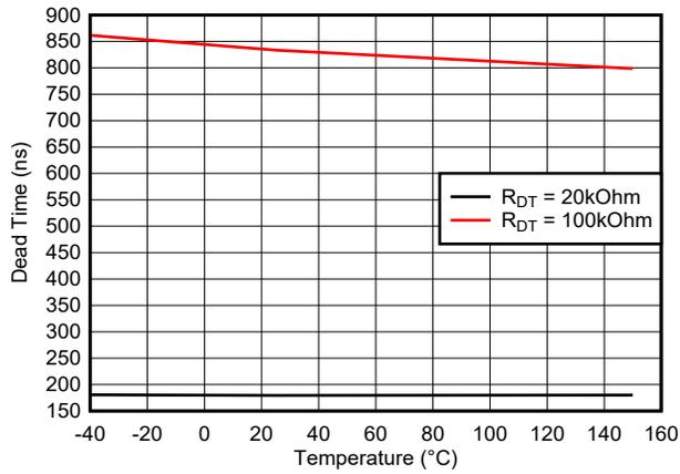
Figure 5-21. Dead Time vs Temperature (with R<sub>DT</sub> = 20 kΩ and 100 kΩ)
