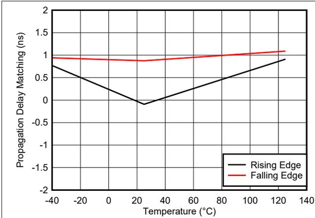
Figure 5-15. Propagation Delay Matching (t<sub>DM</sub>) vs Temperature
