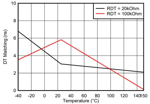
Figure 5-22. Dead Time Matching vs Temperature (with R<sub>DT</sub> = 20 kΩ and 100 kΩ)
