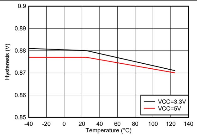
Figure 5-18. IN/EN Hysteresis vs Temperature
