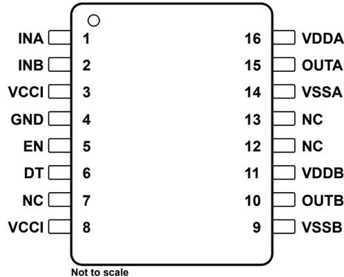
**Figure 4-1. D Package 16-Pin SOIC Top View**
