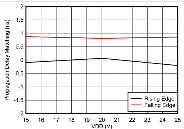
Figure 5-14. Propagation Delay Matching (t<sub>DM</sub>) vs VDD
