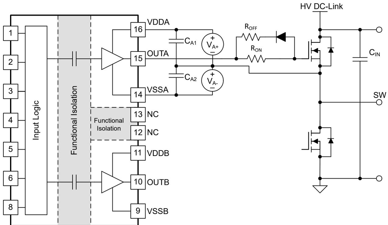
**Figure 8-3. Negative Bias with Two Iso-Bias Power Supplies**
