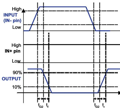
(PWM Input to IN- Pin (IN+ Pin Tied to VDD))
