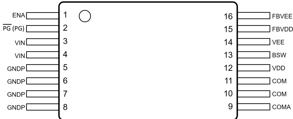
Figure 5-1. DHA Package, 16-Pin SSOP (Top View)
