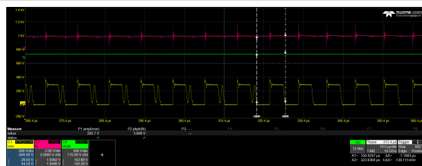
Figure 8-2. 1st and 2nd Valley Operation at 115VAC
