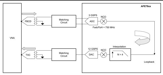
Figure 1-2. ADC to DAC Low Latency Loopback
