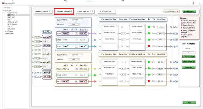
Figure 2-3. ADC to DAC JESD Loop Back Enable Mode
