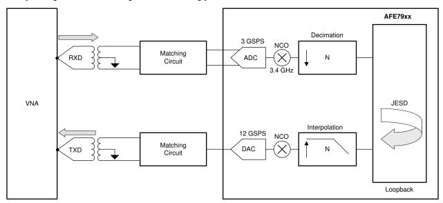
Figure 1-1. ADC to DAC JESD Loopback
