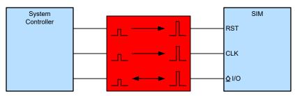
Figure 8-1. Example SIM Card Voltage Translation Block Diagram
