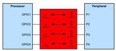
**Example GPIO Voltage Translation Block Diagram**
