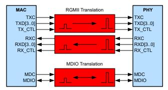
Figure 7-1. Example MAC to PHY Voltage Translation Block Diagram
