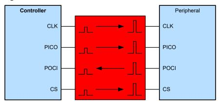
**Example SPI Voltage Translation Block Diagram**
