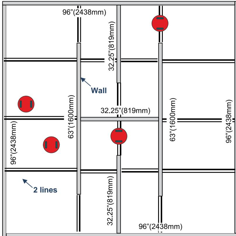
Figure 11. Create a robot explorer that races around a track with bump sensors, line sensors, and IR sensors. Multiple robots can race at the same time. The lines are perpendicular to walls. Each line marking is has two lines (thick and thin) so robot can measure angle and direction.
