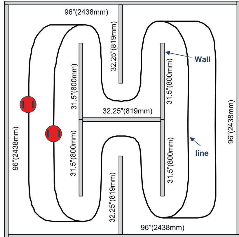
Figure 12. Create a robot explorer that races around a track with bump sensors and line sensors.
