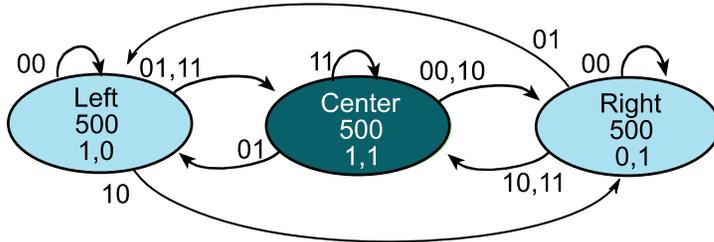
Figure 14. Moore FSM state graph to implement line following. The time in each state is shown in 1ms units.
