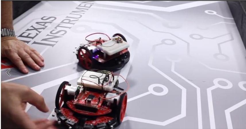
Figure 13. The robots with the microphones will dance to the sounds generated in the robot with the speaker.
