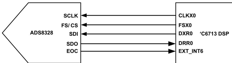
**Figure 1. Hardware Connection**
