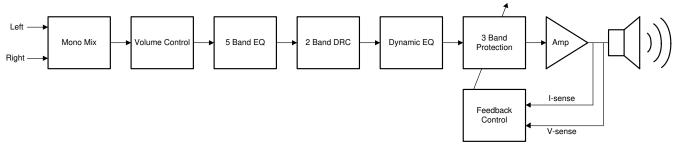
Figure 2-12. Smart Amp Signal Chain
