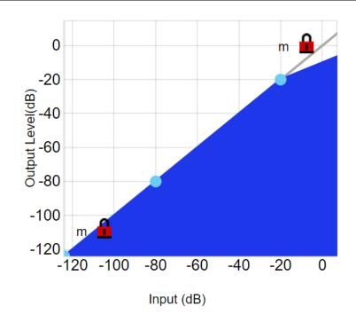
Figure 2-21. DRC Compression Ratio Curve
