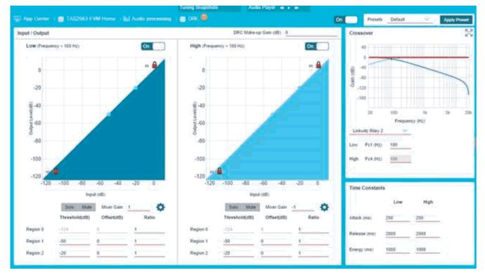
Figure 2-17. 2-Band DRC Control
