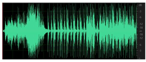
Figure 2-20. Typical Compression Sequence for Optimal Loudness—DRC Output, Compressed With Makeup Gain
