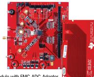
TI ADC Evaluation Module with FMC-ADC-Adapter Connection to Xilinx Evaluation Kit
