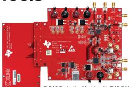
TI DAC Evaluation Module with FMC-DAC-Adapter Card Connection to Xilinx Evaluation Kit
