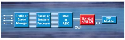
Figure 1: XFP-based Line Card
