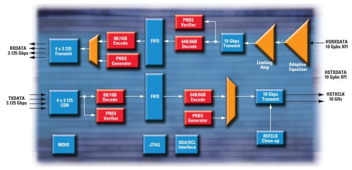
Figure 2: TLK10021 Block Diagram
