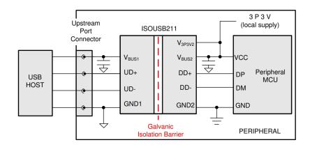
Example: Provide High-Voltage Protection and Enhanced Signal Integrity for USB 2.0
