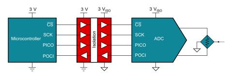
**Example SPI Isolation Block Diagram**
