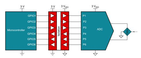
**Example GPIO Isolation Block Diagram**
