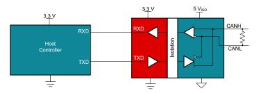
**Example CAN Isolation Block Diagram**
