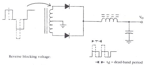
$$= 2R \left[ \frac{V_0}{(T - t_d)/T} + V_F \right] + \text{ leakage inductance spike} \qquad \frac{(T - t_d)}{T} = 0.9 \text{ to } 0.95$$
