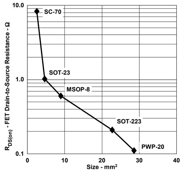
Fig. 6.  $R_{DS(on)}$  variability by package-size.
