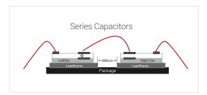
Transferring signals using SiO<sub>2</sub> isolation capacitors.
