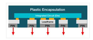
HotRod<sup>™</sup> packaging eliminating bond-wires while maintaining excellent thermal performance.
