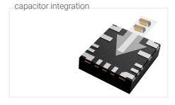
Reducing radiated noise by in-package high-frequency capacitor integration.
