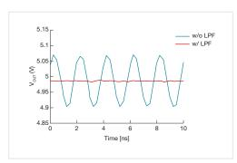
High PSRR enable better filtering and lower output noise.
