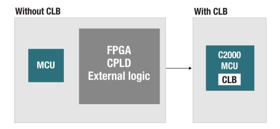
C2000 Configurable Logic Block (CLB) enables customization in a microcontroller based real-time control system while eliminating or reducing the size of the FPGA, CPLD, or external logic
