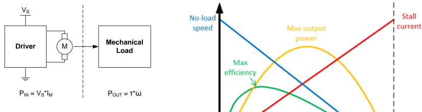
Electrical power is converted into mechanical power
