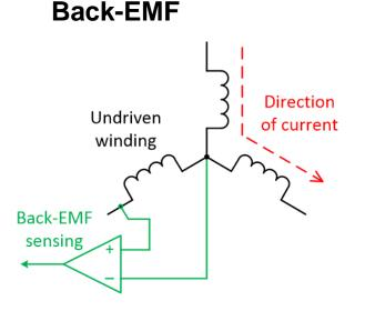
Figure out where the motor is through Back-EMF
