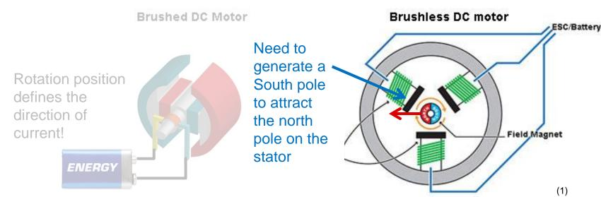
Commutator reverses flow of current to make sure that the magnetic field generated on the rotor is always opposed by the field on the stator
