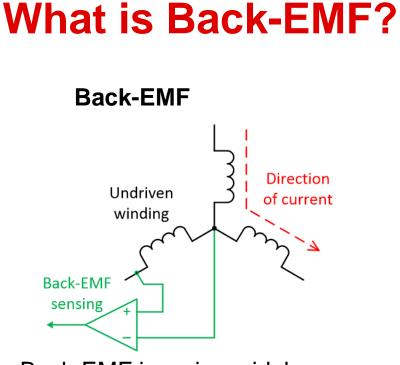
Back-EMF is a sinusoidal or trapezoidal voltage generated on the motor while it is spinning
