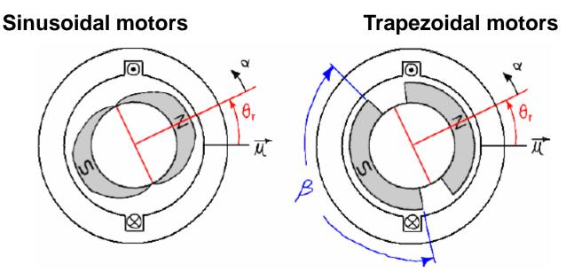
Ideally driven with a sinusoidal current
