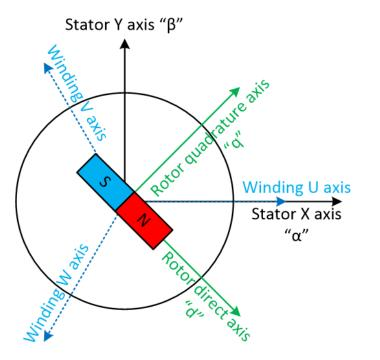
FOC applies all motor torque perpendicular to the rotor
