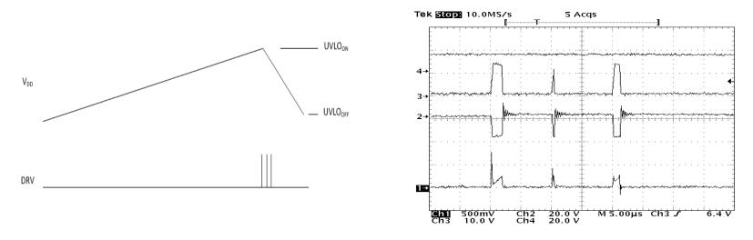
> At UVLO<sub>ON</sub> three gate drive pulse are initiated:
