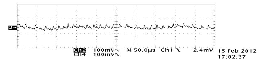
> Frequency jitter does cause a small amount of low frequency output ripple
