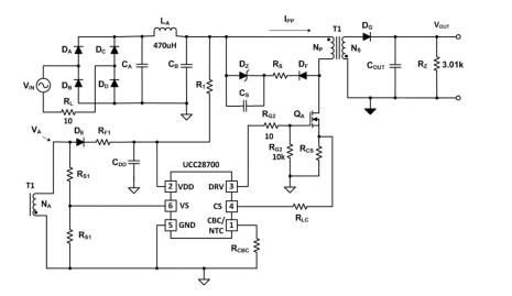
$C_{OUT1} \ge \frac{I_{MAX}}{dV \times f_{min}}$
