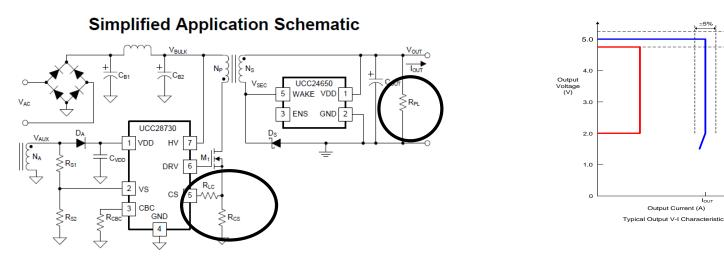
> R<sub>CS</sub> and R<sub>LC</sub> adjusted to fine tune circuit for maximum current (I<sub>OCC</sub>)  $\succ$  Preloading (R<sub>PI</sub>) is added/adjusted
