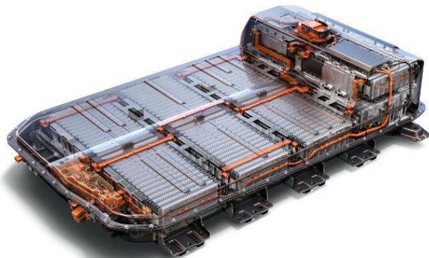
Chevy Bolt 60 kWh 350 V
