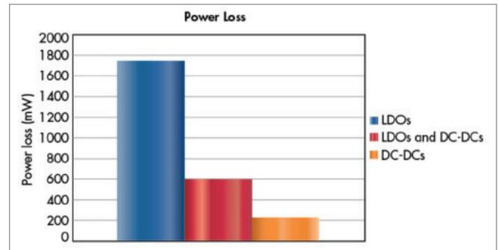
Using just dc-dc converters is sometimes more expensive than using just LDOs, due to the generally higher device cost and additional passives that are required. This depends on the exact LDO and dc-dc required by the specific data converter.
