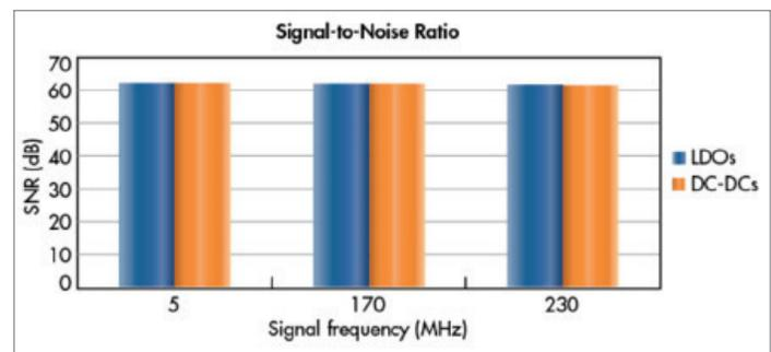
The LDOs provide acceptable noise performance for the ADC and serve as the baseline case for comparison. LDOs are usually the lowest-cost solution for a 12-bit data converter due to the low device cost, as well as low number and cost of passive components. Higher-resolution data converters typically require much-higher-performance LDOs, which are more expensive.
