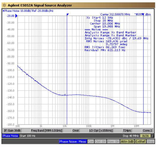
Figure 3. LMK61E2 312.5 MHz Phase Noise
