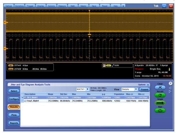
Figure 2. Unfiltered TIE Measurement Results
